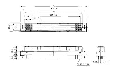
Note: The PCB mounting pattern is equivalent to PCN10-\*S-2.54DSA.
