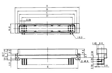
The 48 contact type contains guide key grooves at 8 points.
