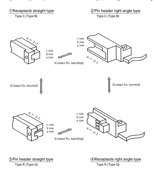
Note: The DIN connector is basically standardized in combination with straight and right angle types. As shown above in illustrationss;
