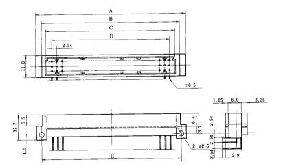
The 48 contact type contains guide key grooves at 8 points.
