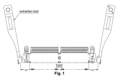
Step 2 Pull out the transmission module holding the tools straight.
